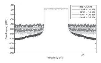
**Fig. 13.** Spectrum of the GFDM signal before and after passing through the AWGN channel for different SNRs
