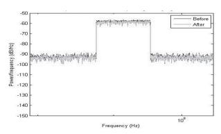
**Fig. 14.** GFDM signal after passing through the Rayleigh channel
