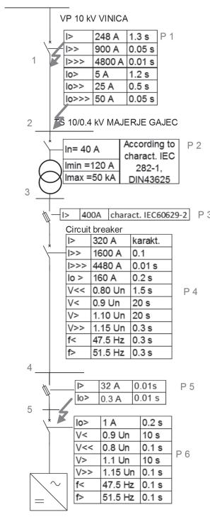
**Fig. 8.** A simplified single-line diagram of the PV power plant and proposed protection settings
