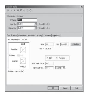
Fig. 3. Inverter characteristics, specification tab
