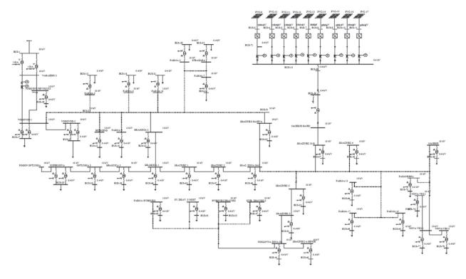
Fig. 5. Model of the observed 10 kV distribution network
