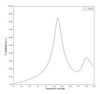
**Fig. 7.** Frequency response when the capacitor bank is switched on
